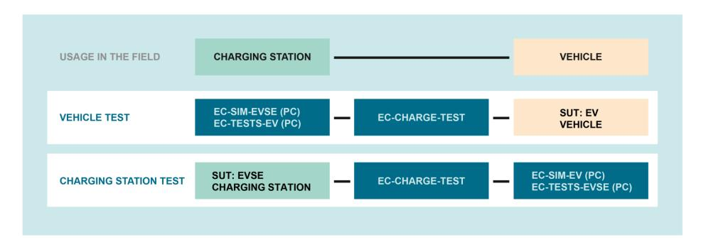
The solutions are based on the DIN 70121 and ISO 15118 charging standards for power line communication (PLC).
